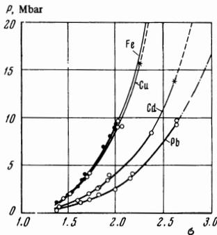
FIG. 3. Shock adiabats of copper, cadmium, lead, and iron at pressures up to 20 Mbar: \* - our results; ○, ●, and thick lines - absolute values of the dynamic compressibility taken from [1<sup>3</sup>, 5]; thin continuous lines - relative compressibilities of metals (the shock adiabat of iron is taken from [4]); chain curve - interpolated adiabat of lead according to [4]; dashed curves are the extrapolated parts of the dynamic adiabats of copper and cadmium.
