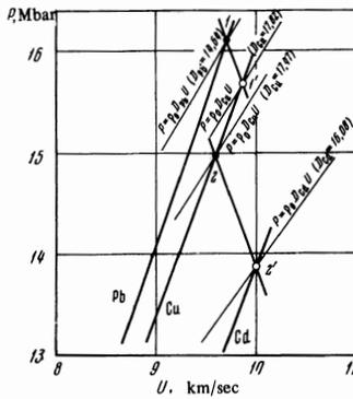
FIG. 2. Determination of the shock-compression parameters of copper and cadmium by the reflection method. ●: 1, 2) Initial states of shock-compressed lead and copper samples; 1-1', 2-2') expansion curves of lead and copper. ○: 1', 2') shock-compressed states of copper and cadmium (D in km/sec).
