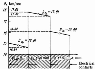
FIG. 1. Schematic representation of the samples and the results of measurements of the wave velocities (in km/sec) in lead, copper, and cadmium. O represents experimental points.
