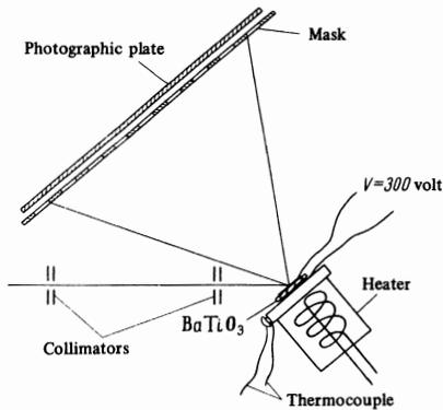
FIG. 3. Schematic diagram of the experiment.
