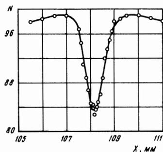
FIG. 7. The dependence of the blackening density of the photographic emulsion (in relative units) on the coordinate of the photometered section (according to the microphotometer scale) on crossing the shadow of the  $\{110\}$  plane.
