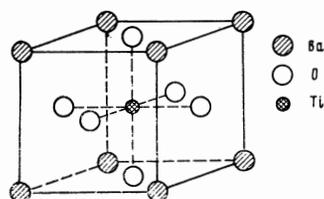
FIG. 1. The unit cell of barium titanate (BaTiO<sub>3</sub>).
