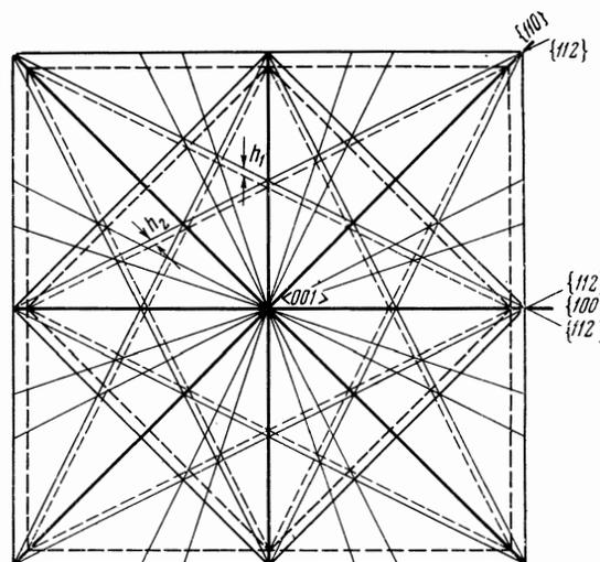
FIG. 2. Schematic distribution of lines of intersection of the crystallographic planes of the barium titanate lattice with the plane of the photographic plate. The continuous lines correspond to the cubic phase (T > 120°C), the dashed lines — to the tetragonal phase (T < 120°C).
