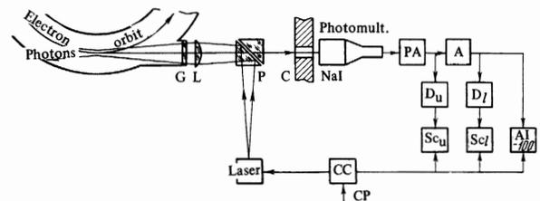
FIG. 1. Block diagram of experimental setup. G – glass, L – lens, P – prism, C – collimator,  $D_l$  and  $D_u$  – discriminators, AI – 100 – pulse analyzers,  $Sc_l$  and  $Sc_u$  – scaler circuits, CC – control circuit CP – control pulse.
