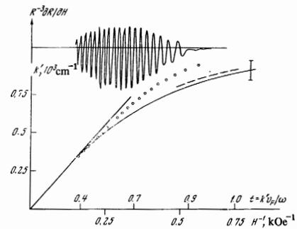
FIG. 2. Spectrum of the wave for strong spatial dispersion. Points—data of experiment for 9.62 GHz,  $\mathbf{k} \parallel \mathbf{C}_2$ ,  $\mathbf{H} \perp \mathbf{C}_3 \parallel \mathbf{J}$ ,  $\varphi = 4^\circ 40'$ . Continuous curve—calculation for  $\omega/\Omega \ll 1$ , dashed curve—with account of the correction for time dispersion. Straight line—asymptote as  $H^{-1} \rightarrow 0$ . The vertical bar indicates the accuracy of the calculation.
