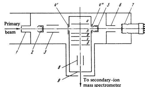
FIG. 1. Collision chamber and system for forming secondary-ion beams.
