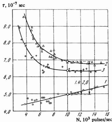
Measurements of  $\Delta\tau$  (correlation) in Xe and Ne. 1—resolving time of the coincidence circuit; 2—correlation in Xe, and 3—correlation in Ne under the same geometrical experimental conditions.
