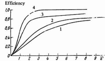
FIG. 2. Dependence of the energy coefficient of conversion of a frequency doubler (i.e., efficiency equal to  $W_2/W_{10}$ ), excited by a laser pulse or by single mode radiation, on the reduced length  $z' = z(l_q^{-1} + l_\sigma^{-1})$  for different values of  $C = (l_q/l_\sigma)^2$ : curve 1 — 0.5, 2 — 1.0, 3 — 10. For single-mode laser radiation  $z' = z(l_a^{-1} + l_\sigma^{-1})$ ,  $C = (l_a/l_\sigma)^2$ . Curve 4 corresponds to conversion of plane monochromatic radiation.
