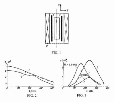
the difference between the ordinates by  $\Delta \epsilon$ . Figure 3 shows the curves for  $\Delta \epsilon$  (f) at different values of H\_ and P (P = 0.32 Torr for curves 1 and 2, and P = 0.64 Torr for curve 3).
