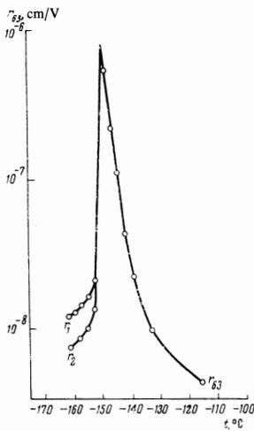
FIG. 1. Electro-optical coefficients  $r_i$  as functions of temperature for the KDP crystal.  $r_{63}$  — at  $T > T_C$ ;  $r_1, r_2$  — at  $T < T_C$ .
