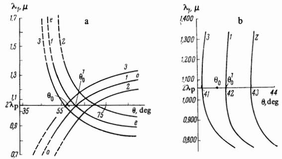
FIG. 2. Shift of the tuning curves following the application of an external field. a — for the (eoe) interaction; b — for the (eoo) interaction.  $\theta_0$  and  $\theta_0^T$  are phase-matching angles for the degenerate case at  $T = 300^\circ\text{K}$  and  $T = T_C$  respectively.
