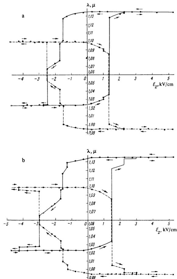
FIG. 9. Wavelength tuning of the parametric laser for two consecutive polarization reversal cycles of the crystal at  $T < T_C$  ( $T = 109^\circ\text{K}$ ). a - 1st cycle; b - 2nd cycle. Arrows indicate the cycling direction.
