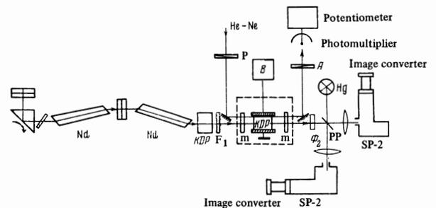
FIG. 3. Diagram of the experimental setup.  $F_1$  — liquid filter;  $F_2$  — KS-10 filter; B — high-voltage supply; PP — plane-parallel glass plate; P — polarizer; A — analyzer.
