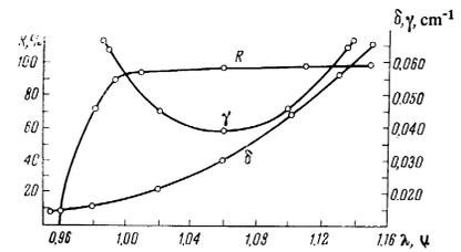
FIG. 6. Dependence of  $R$ ,  $\delta$ , and  $\gamma$  on the wavelength.  $\delta$  — is damping decrement of the KDP crystal and  $\gamma$  is a quantity proportional to  $\sqrt{P_{\text{thr}}}$  [1].
