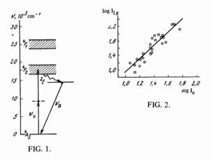
level  ${}^{4}F_{2}$ . Single-quantum absorption of radiation with frequency 9400 cm<sup>-1</sup> by Cr ions in ruby is not observed; thus, a stepwise mechanism of exchange is excluded. With the powers that we used we observed no generation of the second harmonic of the exciting radiation in crystals of ruby and leucosapphire, so that the process of excitation by the harmonic is likewise excluded.
