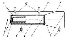
FIG. 2. Dewar for temperature measurements of the absolute cross sections of Raman scattering of light in powders: 1, 6-quartz windows, 2-cell with substance, 3 and 7-tubes for pumping out the air, 4-me-tallic cylinder, 5-diaphragm to limit the aperture of the emerging radiation, 8-vacuum test tube, 9-vacuum jacket, 10-tubes for the inflow and outflow of nitrogen and for the thermocouples, 11-brass insert.
