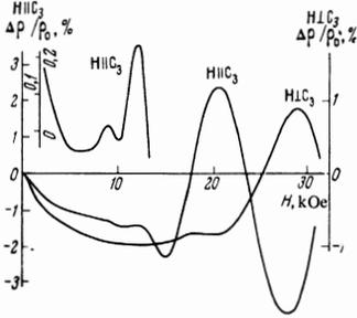
FIG. 2. Dependence of the transverse magnetoresistance of tellurium on the intensity of the field at 1.5°K for one of the samples of transverse orientation. In the upper corner the initial part of the curve for the case  $H \parallel C_3$  is shown in enlarged form with the linear dependence on the field subtracted out.
