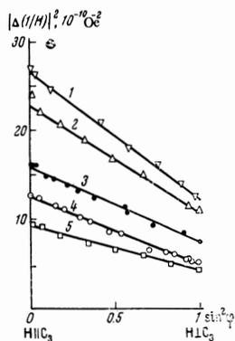
FIG. 6. Dependence of period of oscillation (in the scale of the reciprocal field) on  $\sin^2 \varphi$ . The straight lines correspond to Eq. (2),  $T = 1.5^\circ \text{K}$ .
