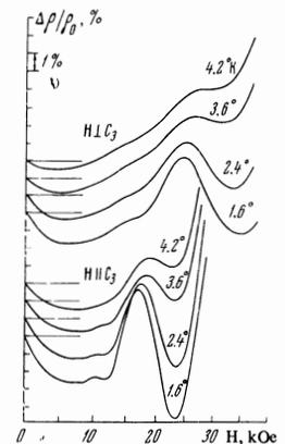
FIG. 1. Dependence of the transverse magnetoresistance ( $I \perp H$ ) of a single crystal of tellurium — sample No. 3 — on the intensity of the magnetic field for two directions of the field and various temperatures.
