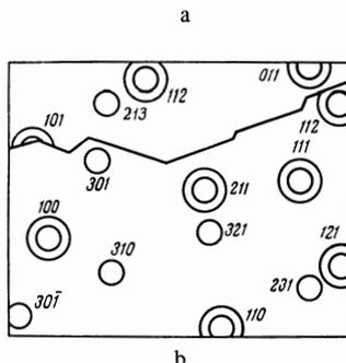
FIG. 1. Intergranular boundary (designated by arrows). The disorientation angle is  $40^\circ$  relative to the [110] axis. Microsteps with height from 3 to 30 Å are located along the boundary.
