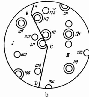
FIG. 2. Recrystallized tungsten bicrystal. Within the limits of the field of view, the boundary consists of two parallel sections (AB and CD) located in the (114) plane, and a transition section BC representing a step of height 150 Å. On section BC, the coincidence of the sites is characterized by  $\sigma = 3$ ; on the remaining sections  $\sigma = 1$ .
