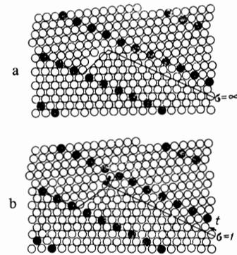
FIG. 4. a—arrangement of atoms near incoherent boundary ( $\sigma = \infty$ ); b—restoration of coherence as a result of partial dislocation.
