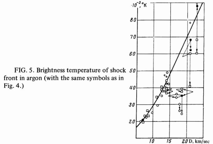
FIG. 5. Brightness temperature of shock front in argon (with the same symbols as in Fig. 4.)
