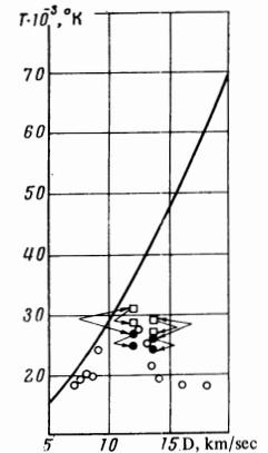
FIG. 7. Brightness temperature of shock front in a mixture of argon and air. The air admixture was 5% for the measurements in the ultraviolet and yellow regions. The curve represents the calculated post-shock temperature for argon. The brightness temperature for blue light was not measured at 45°. Otherwise the symbols are as in Fig. 4.
