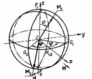
FIG. 1. Diagram illustrating the change of equilibrium configuration of the sublattices on increase of the field  $\mathbf{H}$ , applied in a direction perpendicular to the EA (in an antiferromagnet with nonvanishing DI).
