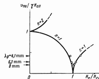
FIG. 6. Dependence of AFMR frequency on magnitude of the field, perpendicular to the easy axis of  $\alpha\text{-Fe}_2\text{O}_3$ . The curves  $n = 1$  and  $2$  are plotted according to formulas (20) and (21) with  $\theta = \pi/2$  and with the values  $H_{C\parallel} = 63 \pm 3 \text{ kOe}$ ,  $H_{C\perp} = 128 \pm 4 \text{ kOe}$  ( $\lambda_p$  is the operating wavelength of the microwave spectrometer).
