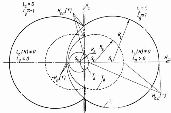
FIG. 2. Phase diagrams in the  $(H_x, H_z)$  plane for an easy-axis antiferromagnet with DI at different temperatures  $T_1 < T_2 < T_3$  and in the case  $H_A \ll H_D \ll H_E$ . The curve  $T_1$  was drawn for the value  $H_{cL}/H_{cH} = 2.1$  characterizing  $\alpha\text{-Fe}_2\text{O}_3$  at  $77^\circ\text{K}$ .
