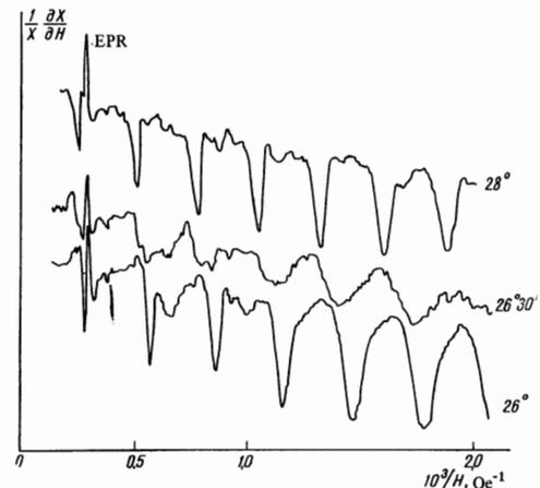
FIG. 3. Resonances in a plane close to (001) in sample IV (cf. table). The angles of inclination of the field to the plane of the sample,  $\varphi$  ( $H$ , [110]) =  $41^\circ - \varphi$ , are given to the right of each curve.
