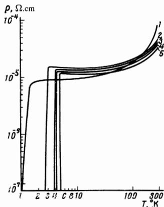
FIG. 1. Temperature dependence of the resistivity of alloys of the W-Re-C system. 1) WC; 2) WC + 1 at.% Re; 3) WC + 2 at.% Re; 4) WC + 4 at.% Re; 5) WC + 6 at.% Re.
