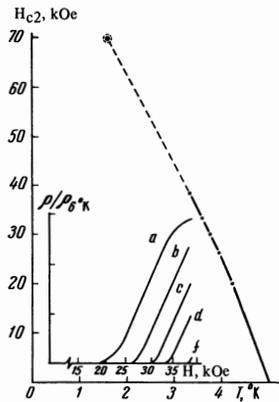
FIG. 4. Temperature dependence of the critical field  $H_{C2}$  of the WC + 6 at.% Re alloy ( $I \approx 3 \text{ A/cm}^2$ ) and the dependence of the reduced resistivity  $\rho/\rho_0$  on the magnetic field intensity at various temperatures ( $^\circ\text{K}$ ): a) 4.2; b) 3.97; c) 3.77; d) 3.6; f) 3.35.
