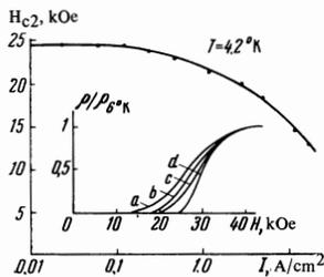
FIG. 5. Dependence of the longitudinal critical field  $H_{C2}$  on the current density  $I$  for the WC + 6 at.% Re alloy at  $T = 4.2^\circ\text{K}$  and the dependence of the reduced resistivity  $\rho/\rho_0$  on the field  $H$  for various values of the current density ( $\text{A/cm}^2$ ): a) 11.7; b) 5; c) 2.7; d) 0.1.
