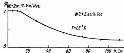
FIG. 7. Dependence of the reduced magnetic moment of the alloy WC + 2 at.% Re on the intensity of an external magnetic field at  $T = 1.5^\circ\text{K}$ .
