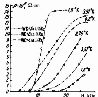
FIG. 3. Dependence of the resistivity of alloys of the W-Re-C system on a transverse magnetic field at various temperatures for a measuring current density  $I = 2$  A/cm<sup>2</sup>.
