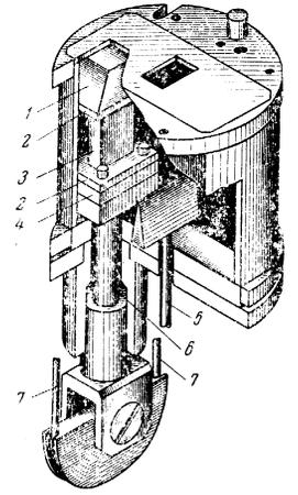
FIG. 1.  $H_{101}$  resonator permitting application of pressure perpendicular to the direction of the external magnetic field.
