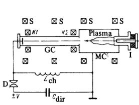
FIG. 1. Direct-discharge circuit: S – solenoid of leading magnetic field (length 5 m, diameter 1 m), MC – metallic vacuum chamber (length 3 m, diameter 25 cm), GC – glass chamber (length 175 cm, diameter 10 cm), K1 – mirror coil No. 1, K2 – mirror coil No. 2, I – coaxial plasma injector D – vacuum discharge gap.
