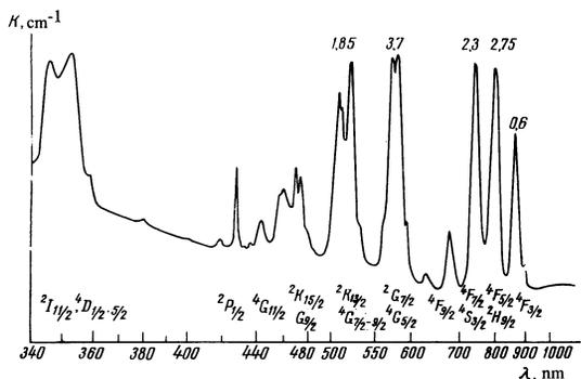
FIG. 2. Absorption spectrum of LaF<sub>3</sub>-Nd<sup>3+</sup> (1%) crystal at 300°K.
