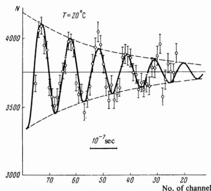
FIG. 3. Muonium precession curve in crystalline quartz. Horizontal axis – number of channel (10.1 nsec wide); vertical axis – counts corrected for exponential decay of meson.
