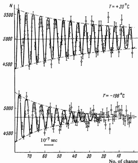
FIG. 4. Muonium precession curves in fused quartz at different temperatures, with 18.5-nsec channel width.
