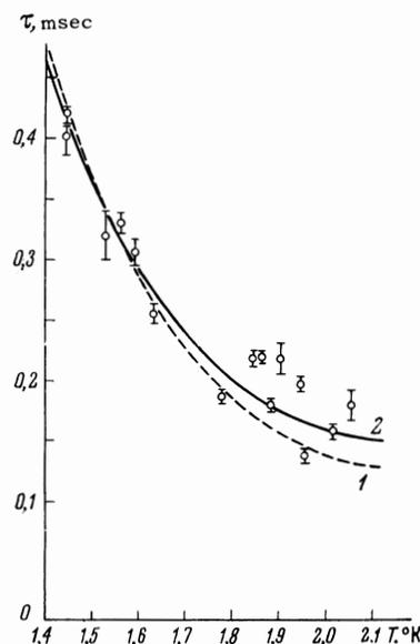
Temperature dependence of the relaxation time in praseodymium ethyl sulfate. Experimental points are data of Griffiths and Glättli; <sup>[17]</sup> curves 1 and 2 are calculated from Eq. (3) for different values of  $R$ .
