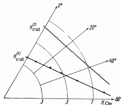
FIG. 3. Dependence of  $H_{\text{cut}}^{(1)}$  and  $H_{\text{cut}}^{(2)}$  on the direction of the magnetic field. The angle is calculated from the plane of the sample.
