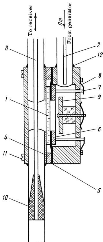
FIG. 1. Diagram of the apparatus for the observation of the transparency of a crystal. 1 – crystal specimen, 2 – input coaxial line, 3 – output coaxial line, 4 – ring gasket of thickness 250 microns, 5 – copper diaphragm of thickness 20 microns, 6 – clamping ring, 7 – polystyrene post, 8 – bronze spring, 9 – resonant strip, 10 – absorber, 11 – clamping screw, 12 – soldering with non-superconducting solder.
