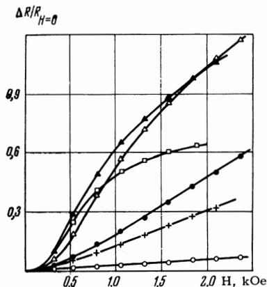
FIG. 4. Relative change in the resistance of sample No. 12 as a function of a longitudinal magnetic field and temperature.  $\circ$  – 4.2°K,  $+$  – 3°K,  $\bullet$  – 2.75°K,  $\Delta$  – 2.5°K,  $\blacktriangle$  – 2°K,  $\square$  – 1.8°K.
