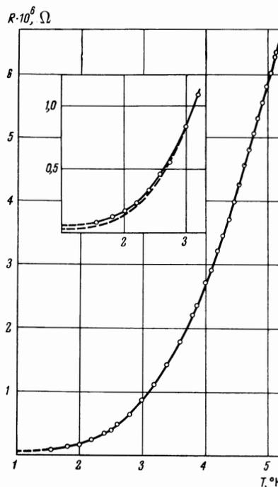
FIG. 2. Dependence of the resistance R on temperature for sample No. 12. The dashed curve shows the dependence of R on T on an enlarged (resistance) scale after subtracting the influence of a longitudinal magnetic field.
