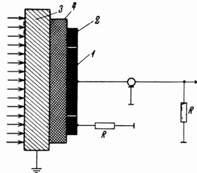
FIG. 1. Experimental setup: 1 – Measuring electrode ( $S = 1 - 12.5$  cm<sup>2</sup>); 2 – guard ring, of area equal to that of the measuring electrode; 3 – screen of metal with known shock adiabat (aluminum, copper); 4 – NaCl sample (thickness  $l_0$  ranges from 0.1 to 0.8 cm). The arrows show the direction of the motion of the shock wave front.
