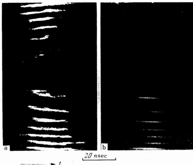
FIG. 4. Streak photograph of the emission spectrum, obtained with 150-mm plate gap in the Fabry-Perot interferometer. The internal fine structure of the lines resulted from the spatial distribution of the emission, not from the structure of the spectrum (lines in the different orders have different structures). a – without a diaphragm inside the resonator, pulse energy 1.2 J; b – with a diaphragm of 0.7-mm diameter inside the resonator, pulse energy 0.2 J.
