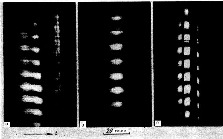
FIG. 3. Streak photograph of two-hole interference pattern. a – 1.2-mm hole separation, in resonator with 0.7-mm diameter diaphragm, pulse energy 0.02 J; c – 0.3-mm hole separation, without diaphragm, pulse energy 0.6 J.
