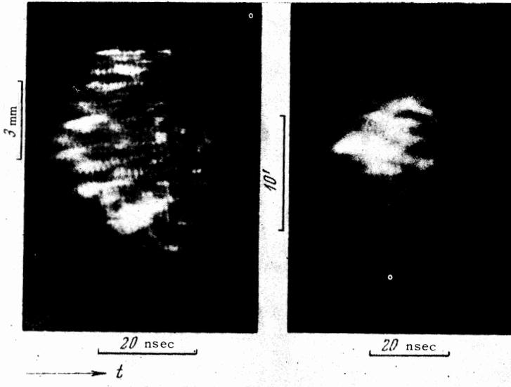
FIG. 1. Streak photograph of radiation field pattern. a – near-field (crystal end face), pulse energy 1.2 J; b – far-field (directional distribution), pulse energy 1.2 J.
