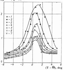
FIG. 4. Dependence of  $\chi_p$  on  $(T - \Theta)$  in field 260 Oe for iron garnets of: 1, Y; 2, Sm; 3, Eu; 4, Er; 5, Gd; 6, Dy; 7, Tb.
