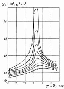
FIG. 3. Dependence of  $\chi_p$  on  $(T - \Theta)$  for Tb iron garnet: curve 1, H = 260 Oe; 2, 390 Oe; 3, 520 Oe; 4, 660 Oe; 5, 790 Oe; 6, 920 Oe; 7, 1050 Oe; 8, 1180 Oe.
