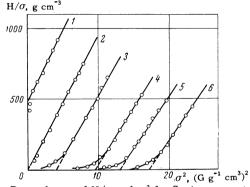
FIG. 1. Dependence of H/ $\sigma$  and  $\sigma^2$  for Sm iron-garnet: curve 1, t = 290.8°C; 2, 289.0°C; 3, 287.4°C; 4, 286.0°C; 5, 284.8°C; 6, 283.4°C.
