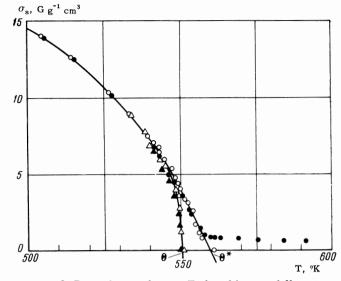
FIG. 2. Dependence of  $\sigma_s$  on T, found by two different methods:  $\Delta \blacktriangle$ , from curves  $H/\sigma = f(\sigma^2)$  for single-crystal and polycrystalline specimens of yttrium garnet;  $O \bullet$ , from curves  $\sigma(H)$  for the same specimens.
