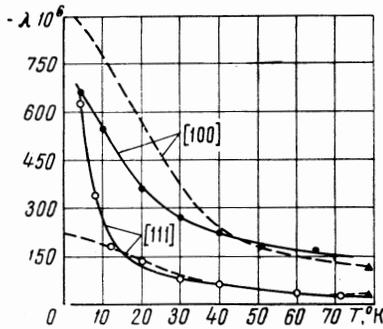
FIG. 4. Temperature dependence of the magnetostriction of single-crystal holmium iron garnet: dashed line – theoretical data ( $H = 0$ ); solid lines – experimental data ( $H = 23$  kOe); ▲ – experimental data from [3].
