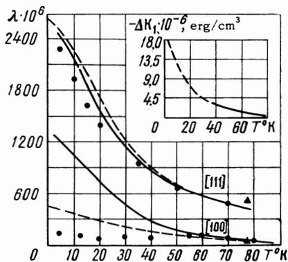
FIG. 2. Temperature dependence of the magnetostriction of terbium iron garnet and of the magneto-elastic contribution ( $\Delta K_1$ ) to the magnetic-anisotropy energy. Dashed lines - theoretical data ( $H = 0$ ); solid lines - experimental data ( $H = 23$  kOe):  $\bullet$  - experimental data ( $H = 0$ ),  $\blacktriangle$  - experimental data of<sup>[2]</sup>.
