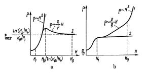
Dependence of the resistance on the intensity of the magnetic field in metals with closed Fermi surfaces: a - number of electrons and holes compensated  $(n_1 = n_2) b - number$  of electrons not equal to the number of holes  $(n_1 \neq n_2)$ . Curves  $1 - for a \neq \pi/2$ , curves  $2 - for a = \pi/2$ .
