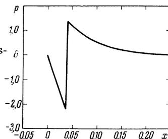
FIG. 9. Distribution of pressures in the presence of a reflected wave.
