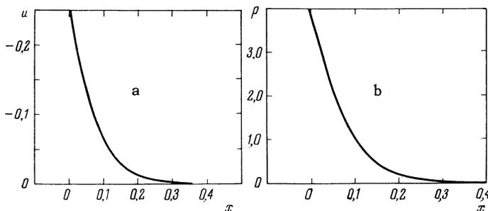
FIG. 8. Distribution of velocities (a) and pressures (b) at the instant  $t_1 = 0.0690$  (emergence of wave to the left boundary).
