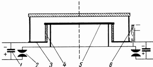
FIG. 1. Diagram of gas-discharge chamber: 1 – Capacitor bank, 2 – vacuum switch, 3 – chamber housing, 4 – porcelain insulator, 5 – anode, 6 – ohmic divider.
