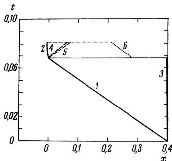
FIG. 6. Plot of shock-wave motion (from right to left), of the free and compressed boundaries, and of the characteristics bounding the compression wave.
