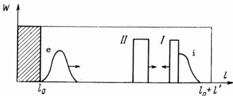
FIG. 2. Observations of induction (i) and echo (e) in a combination sample with account of reflected signals.  $l_0$  is the sample length with impurity centers,  $l'$  the length of the additional sample without impurities ( $l' > v_0 t_1$ ). The remaining notation is the same as in Fig. 1.
