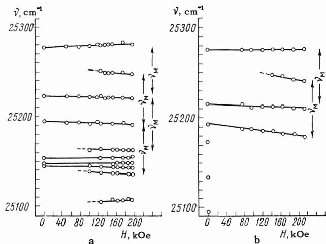
FIG. 1. Dependence of the frequencies of the absorption bands on the strength of the magnetic field ( $T = 20.4^\circ\text{K}$ ): a— $\text{RbMnF}_3$ , b— $\text{KMnF}_3$ . Bands which appear only in fields  $\sim 10^5$  Oe are enhanced with increasing external magnetic fields.
