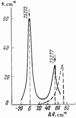
FIG. 3. Shape of the no-magnon and one-magnon bands in the spectrum of  $\text{RbMnF}_3$ ,  $T = 20.4^\circ\text{K}$ . The dashed curve is the calculated shape of the exciton-magnon light absorption band.
