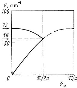
FIG. 5. Spin-wave spectrum in  $\text{RbMnF}_3$  with account of the periodicity of the magnetic structure.
