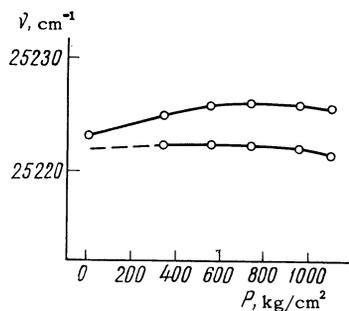
FIG. 6. Splitting of the  $\nu = 25222 \text{ cm}^{-1}$  band in the spectrum of  $\text{RbMnF}_3$  under the influence of a uniaxial deformation;  $T = 20.4^\circ\text{K}$ .
