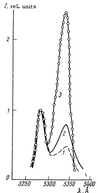
FIG. 3. Spontaneous luminescence spectrum of ZnTe at low current densities  $J_1 < j_2 < j_3 = 0.5 \text{ A/cm}^2$ .
