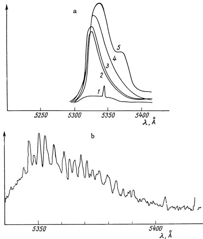
FIG. 2. Stimulated radiation spectrum of ZnTe single crystals. a) Dependence on the excitation current density (sample 1): 1)  $J = 6 \text{ A/cm}^2$ ; 2)  $j = 10 \text{ A/cm}^2$ ; 3)  $j = \text{A/cm}^2$ ; 4)  $j = 14 \text{ A/cm}^2$ ; 5)  $j = 16 \text{ A/cm}^2$ . b) Mode structure of the radiation of ZnTe at a current density of  $25 \text{ A/cm}^2$  (sample 2).
