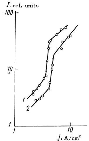
FIG. 1. Dependence of the intensity of radiation  $I$  on the density of the excitation current for two samples of ZnTe.
