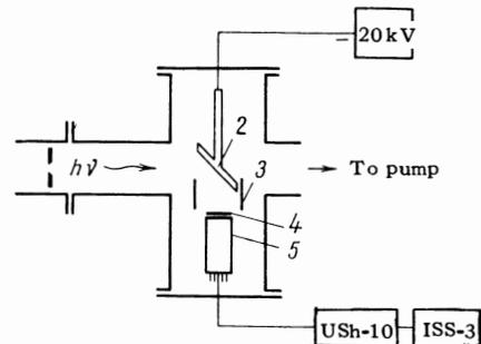
FIG. 2. Scheme of quantum detector. 1—exit slit of vacuum monochromator; 2—converter, 3—focusing electrode, 4—scintillator, 5—photomultiplier FÉU-38.
