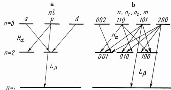
FIG. 3. Level scheme for hydrogen states with  $n = 1, 2$ , and 3: a) in the absence of external fields, and b) in an electric field for which a linear approximation of Stark-effect theory is applicable.
