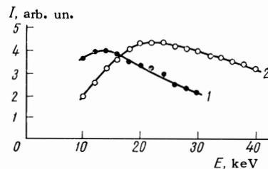
FIG. 9. Excitation functions of the lines (1)  $H_{\alpha}$  and (2)  $L_{\beta}$  for proton-argon charge exchange ( $\mathcal{E} = 600$  V/cm).
