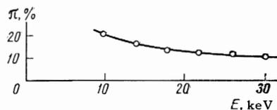
FIG. 10. Polarization of  $H_{\alpha}$  emission induced by proton-argon charge exchange vs. proton energy;  $\pi = (I_{\parallel} - I_{\perp}) / (I_{\parallel} + I_{\perp})$ .
