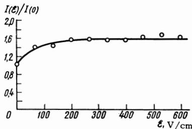
FIG. 1.  $L_\beta$  intensity ratio (with and without a field) vs. external electric field strength for charge exchange between 14-keV protons and He.
