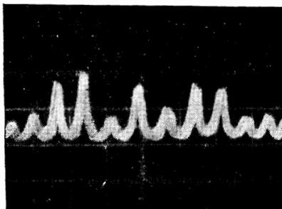
FIG. 2. Spectrum of laser with modulated dielectric constant (200 V applied to the crystal). The emission represents a frequency-modulated signal with  $\sim 3.3$  modulation index.
