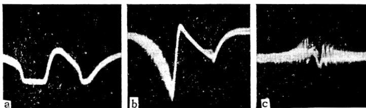
FIG. 3. Dependence of laser light intensity on frequency separation between the modulating signal and intermode beats; this was recorded by oscillograph 6. The modulating frequency increases from right to left. Voltage applied to crystal: a) and b) 200 V; c) 300 V. In case a) the laser was slightly maladjusted.
