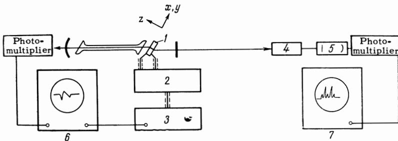
FIG. 1. Block diagram of apparatus. 1—electro-optical crystal, 2—amplifier, 3—rocking-frequency oscillator, 4—optical decoupling and matching lens, 5—scanning interferometer, 6,7—oscillographs (oscillograph 7 was synchronized with the oscillator 3).
