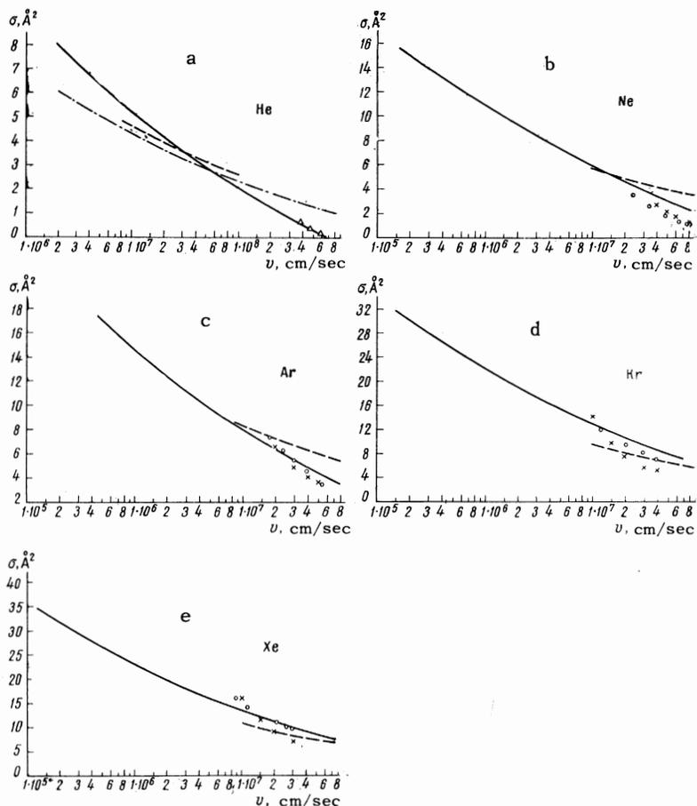
FIG. 2. Cross sections for double resonant charge exchange in inert gases. The solid line shows the result of the present work;  $\triangle$ ,  $\circ$ ,  $\times$  — experimental data from [13], [14], and [15], respectively. Dashed curves—calculation from [7]; dash-dot—calculation from [8].
