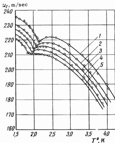
FIG. 1. Temperature dependence of the velocity of first sound: curve 1 — He<sup>4</sup>, 2 — 6.3% He<sup>3</sup>, 3 — 11.05% He<sup>3</sup>, 4 — 15.56% He<sup>3</sup>, 5 — 19.53% He<sup>3</sup> (the molar concentrations are shown);  $\Delta$  — according to [3],  $\square$  — according to [2],  $\circ$  — present research.
