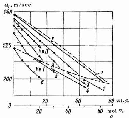
FIG. 2. Dependence of the velocity of first sound on the concentration: curve 1 —  $T = 1^\circ\text{K}$ , 2 —  $1.4^\circ\text{K}$ , 3 —  $1.6^\circ\text{K}$ , 4 —  $1.8^\circ\text{K}$ , 5 —  $2.0^\circ\text{K}$ , 6 —  $3.0^\circ\text{K}$ ; + — according to [1],  $\bullet$  — according to [2],  $\bullet$  — according to [3],  $\circ$  — present research. The dashed curves indicate the  $\lambda$  lines and the S line of the stratification of the solutions.
