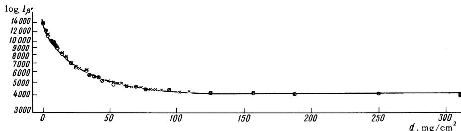
FIG. 2. Intensity of  $\text{Na}^{22}$  radiation reflected from a tin-lead alloy with effective atomic number 73 (calculated by Muller's formulas [4]) and from tantalum (atomic number 73) at different aluminum-filter thicknesses: O - tantalum, x - tin-lead alloy. The  $\gamma$  background was not subtracted from the instrument readings.
