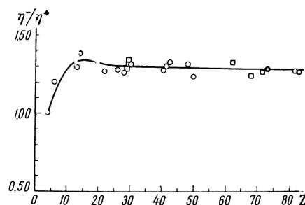
FIG. 1. Ratio of electron reflection coefficient (Tl<sup>204</sup> source) to the positron reflection coefficient (Na<sup>22</sup> source) as a function of the atomic number: ○ — element, □ — alloy.
