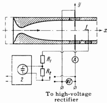
FIG. 7. Schematic diagram of the apparatus used in probe measurements: 1) probe; 2) cathode-ray oscillograph;  $R_1$  and  $R_2$  are measuring resistances.
