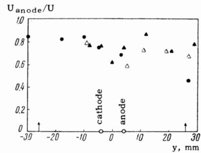
FIG. 8. Distribution of the potential in a steady diffuse discharge:  $\bullet$  -  $x = 47 \text{ mm}$ ;  $\Delta$  -  $x = 90 \text{ mm}$ ;  $\triangle$  -  $x = 120 \text{ mm}$ . Arrows indicate the positions of the cathode and anode bands for  $x \geq 47 \text{ mm}$ .
