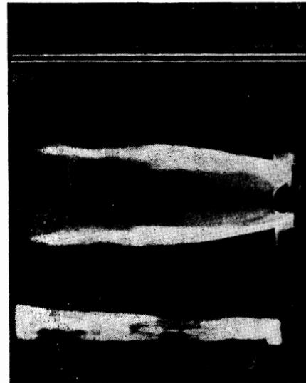
FIG. 6. Current and voltage oscillograms, and photographs of a diffuse discharge. 1) Oscillograms; 2) lateral view; 3) view from top.  $\rho = 0.127 \text{ kg/m}^3$ ,  $l = 8 \text{ mm}$ ,  $v = 600 \text{ m/sec}$ . The relative positions of oscillograms are the same as in Fig. 5. Current amplitude scale: 1 cm = 7.4; voltage amplitude scale: 1 cm = 8 kV.
