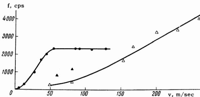
FIG. 4. Dependence of the frequency of the current and voltage fluctuations on the air stream velocity: ● —  $\rho = 1.29$  kg/m<sup>3</sup>;  $l = 1.7$  mm; ▲ —  $\rho = 0.14$  kg/m<sup>3</sup>;  $l = 10$  mm; △ —  $\rho = 0.27$  kg/m<sup>3</sup>;  $l = 10$  mm.
