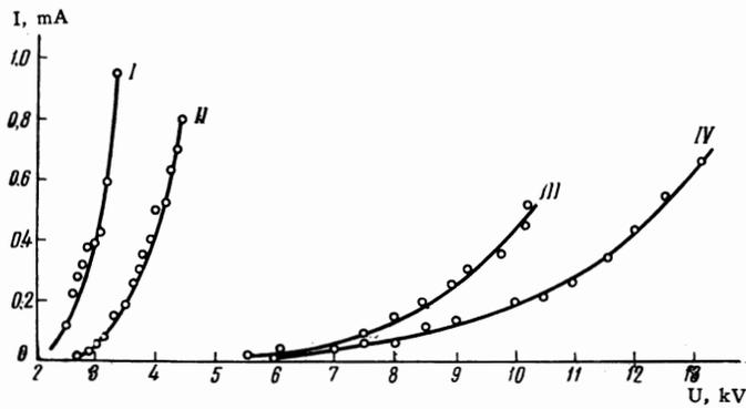
FIG. 1. Current-voltage characteristics ( $I$  in mA) of a pre-breakdown discharge. I)  $l = 10 \text{ mm}$ ,  $\rho = 0.135 \text{ kg/m}^3$ ; II)  $l = 15 \text{ mm}$ ,  $\rho = 0.135 \text{ kg/m}^3$ ; III)  $l = 10 \text{ mm}$ ,  $\rho = 0.54 \text{ kg/m}^3$ ; IV)  $l = 15 \text{ mm}$ ,  $\rho = 0.54 \text{ kg/m}^3$ .
