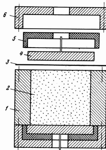
FIG. 1. Resonator (upper part is shown schematically): 1—housing; 2—rouge filter; 3—film; 4—massive electrode; 5—insulation packing; 6—cover.
