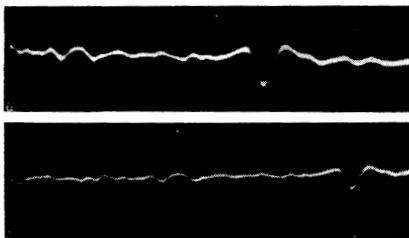
FIG. 3. Pulses of fourth sound in a solution with 11.05%  $\text{He}^3$ : a—temperature 1.60°K; b—temperature 1.85°K. Only the first pulses are shown. The left edge coincides with the start of the sweep.
