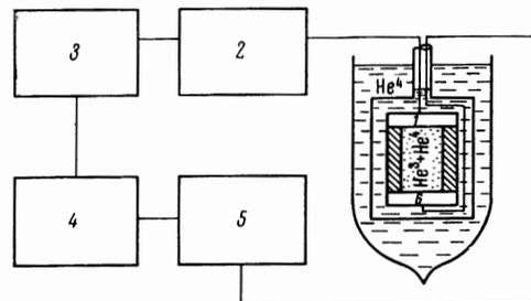
FIG. 2. Measuring apparatus: 1—radiator; 2—blocking generator; 3—paired pulse generator; 4—display unit; 5—amplifier; 6—receiver.
