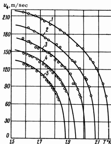
FIG. 4. Temperature dependence of the velocity of fourth sound: curve 1—pure  $\text{He}^4$ ; 2—6.30%  $\text{He}^3$ ; 3—11.05%  $\text{He}^3$ ; 4—15.56%  $\text{He}^3$  (molar concentrations are shown). The solid lines correspond to values computed from Eq. (3).
