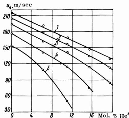
FIG. 5. Isotherms of fourth sound velocity: curve 1— $T = 1.60^\circ\text{K}$ ; 2— $T = 1.70^\circ\text{K}$ ; 3— $T = 1.80^\circ\text{K}$ ; 4— $T = 1.90^\circ\text{K}$ ; 5— $T = 2.00^\circ\text{K}$ .
