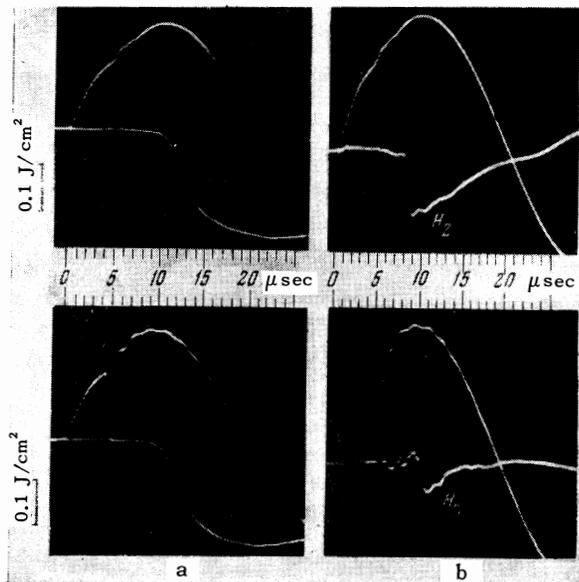
FIG. 6. Oscillograms of the discharge current up to 150 kA (upper curves): (a) signal from a thermal probe, (b) signal from the  $H_z$  field (lower curves). The hydrogen pressure is 0.05 mm Hg; upper curves, without stabilization, lower curves, with stabilization.
