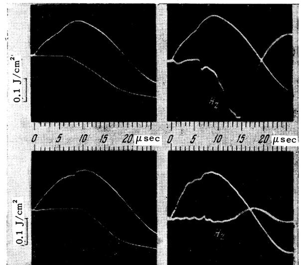
FIG. 5. Oscillograms of the discharge current up to 100 kA (upper curves): (a) signal from a thermal probe, (b) signal from the  $H_z$  field (lower curves). The hydrogen pressure is 0.05 mm Hg; upper curves, without stabilization, lower curves, with stabilization.
