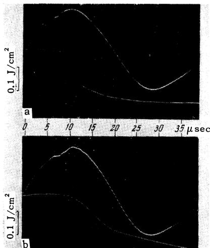
FIG. 4. Signals from the thermal probe (lower curves) taken together with the current in the primary discharge 120 kA (upper curves): (a) without stabilization, (b) with stabilization. The dashed lines show the energy loss to the walls.
