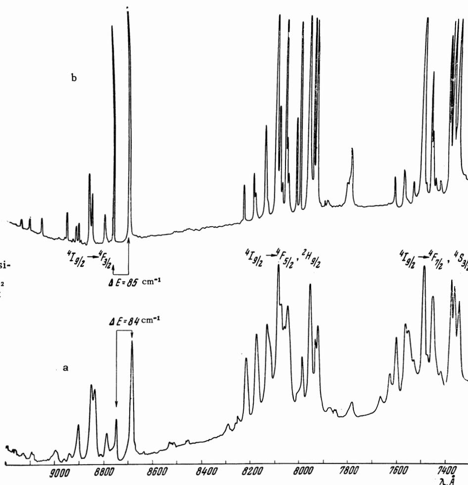
FIG. 2. Absorption spectra of a crystal of  $Y_3Al_5O_{12}-Nd^{3+}$  (0.5%); transitions  ${}^4I_{9/2} \rightarrow {}^4F_{3/2}$ ,  ${}^4I_{9/2} \rightarrow {}^4F_{5/2}$ ,  ${}^2H_{9/2}$  and  ${}^4I_{9/2} \rightarrow {}^4F_{7/2}$ ,  ${}^4S_{3/2}$ . Spectrum a—at 300°K, b—at 77°K.
