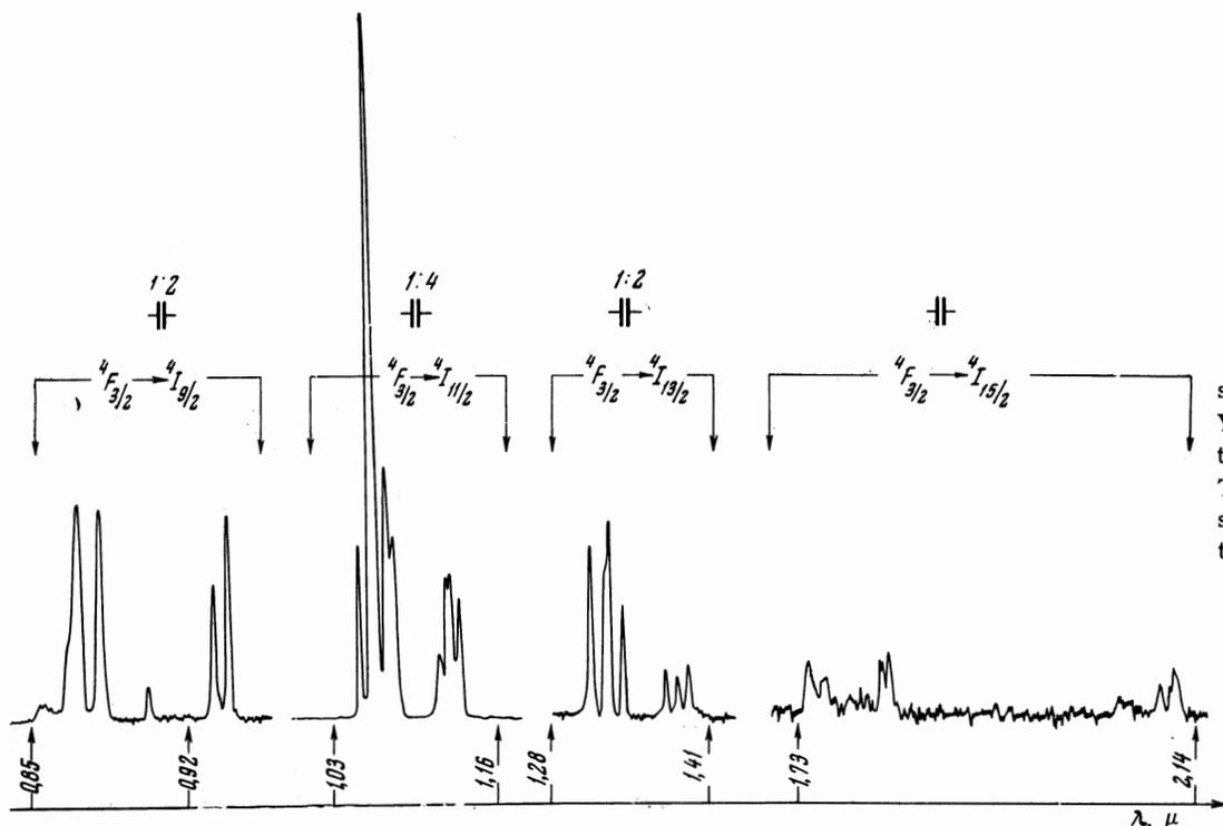
FIG. 4. Luminescence spectrum of crystal of  $Y_3Al_5O_{12}-Nd^{3+}$  (0.5%); transitions  ${}^4F_{3/2} \rightarrow {}^4I_{9/2-15/2}$ ,  $T = 300^\circ K$  (the relative slit widths are given at the top).
