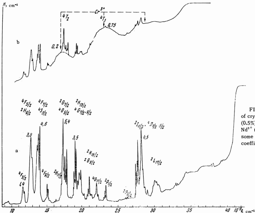
FIG. 1. Absorption spectra of crystals: a—of  $Y_3Al_5O_{12}-Nd^{3+}$  (0.5%), b— $Y_3Al_5O_{12}-Cr^{3+}$  (0.2%)— $Nd^{3+}$  (0.2%);  $T = 300^\circ K$ . For some lines the peak absorption coefficients are shown.
