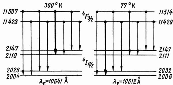
FIG. 7. Diagram of crystal splitting of  $^4F_{3/2}$  and  $^4I_{11/2}$  terms in a  $Y_3Al_5O_{12}-Nd^{3+}$  crystal.
