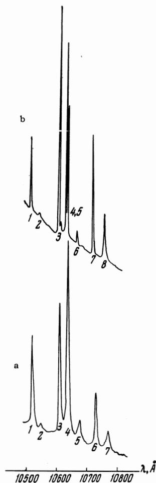
FIG. 5. Luminescence spectra of crystal of  $Y_3Al_5O_{12}-Nd^{3+}$  (0.5%); transition  ${}^4F_{3/2} \rightarrow {}^4I_{11/2}$ . Spectrum a—for  $300^\circ K$ , b—for  $77^\circ K$ .
