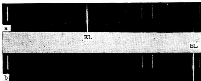
FIG. 6. Emission spectra of crystal of  $\text{Y}_3\text{Al}_5\text{O}_{12}-\text{Nd}^{3+}$  (0.5%): a—for 300° K, b—for 77° K. EL—emission lines.
