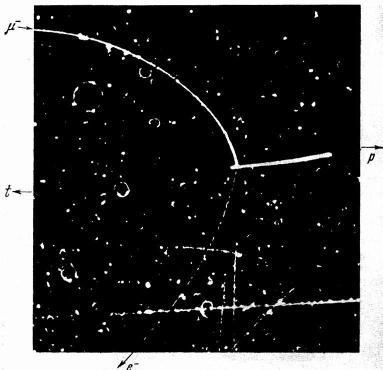
FIG. 3. Photograph of a reaction (3) event.
