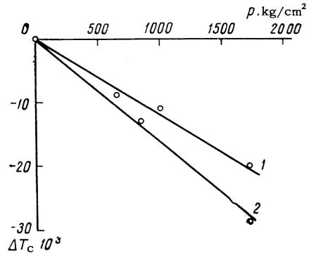
FIG. 5. Pressure dependence of  $\Delta T_c$  of thallium. Curve 1 - thallium with a 3.57 at. % content of indium, 2 - thallium with a 7.15 at. % content of indium.
