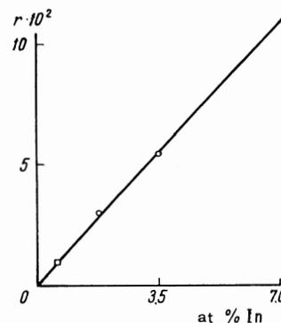
FIG. 1. The residual resistivity  $r = R(4.2^\circ \text{K})/R(300^\circ \text{K})$  of thallium alloys as a function of the indium concentration:  $\circ$  — present work,  $\square$  — data from<sup>[2]</sup>.
