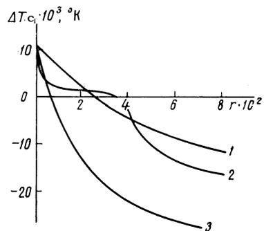
FIG. 6. Dependence of  $\Delta T_c$  of thallium on  $r$  at a pressure of  $1730 \text{ kg/cm}^2$ : curve 1 - thallium with an admixture of bismuth, [1] 2 - thallium with an admixture of antimony, [1] 3 - thallium with an admixture of indium.
