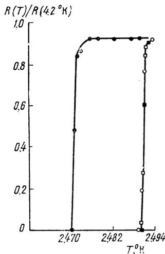
FIG. 2. Superconducting-transition curves of Tl - In alloy with  $r = 3.1 \times 10^{-2}$ . The sample was placed inside a bomb:  $\square$  -  $p = 0$ ,  $\bullet$  -  $p = 1730 \text{ kg/cm}^2$ ,  $\blacksquare$  -  $p = 0$  (after taking off the pressure);  $\circ$  - sample placed outside the bomb.
