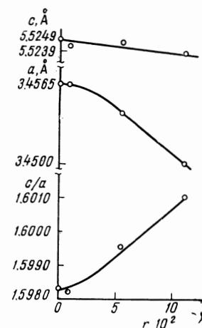
FIG. 7. Dependence of the lattice parameters  $a$  and  $c$  and of the  $c/a$  ratio on the indium concentration.
