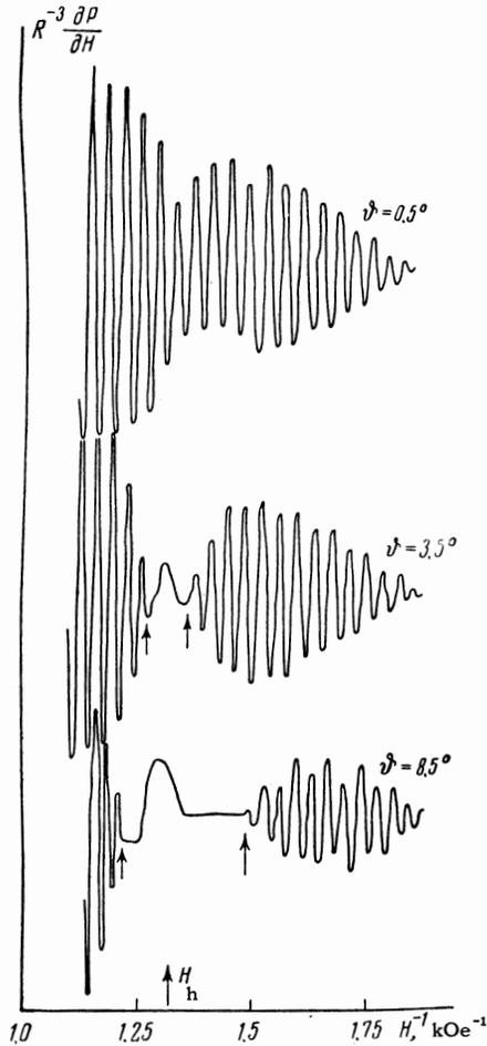
FIG. 3. The recordings from experiments intended to measure the limits of the Doppler damping (Fig. 2,  $D_h^S$ ), indicated by arrows.  $H_h$  is the first-order cyclotron resonance field for holes when  $\vartheta = 0$ .
