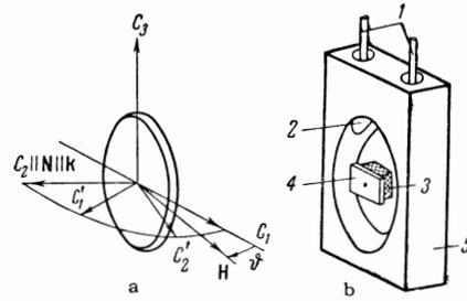
FIG. 1. a) Orientation of the crystallographic axes of bismuth in a disk sample:  $C_3$  – trigonal axis;  $C_2, C_2'$  – binary axes;  $C_1, C_1'$  – bisectrix axes;  $N$  – normal to the sample surface;  $k$  – wave vector of a magnetoplasma wave;  $H$  – magnetic field. b) Schematic representation of the strip resonator structure: 1) – coaxial transmission lines; 2) – coupling aperture (the second aperture is not shown); 3) – foamed polystyrene; 4) – copper resonance strip; 5) – casing.
