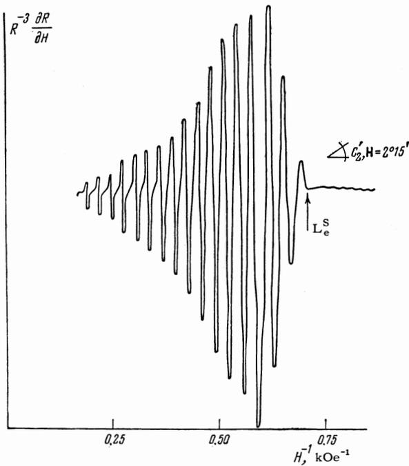
FIG. 7. The recordings from an experiment intended to measure the Landau damping limit  $L_e^S$ . The reduction in the oscillation amplitude as the field increases is not due to the damping of the waves (the width of the peaks decreases).
