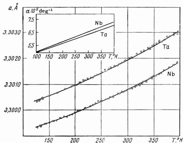
FIG. 1. Temperature dependence of the crystal lattice parameters and linear expansion coefficients of tantalum and niobium.
