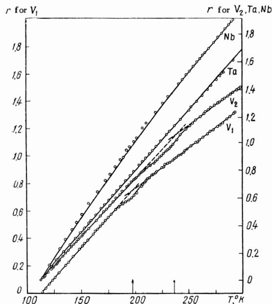
FIG. 2. Temperature dependence of the relative electrical resistance  $r = [R(T) - R(110^\circ\text{K})]/R(110^\circ\text{K})$  of tantalum, niobium, and vanadium ( $V_1$  - 99.74% pure,  $V_2$  - 99.20% pure)
