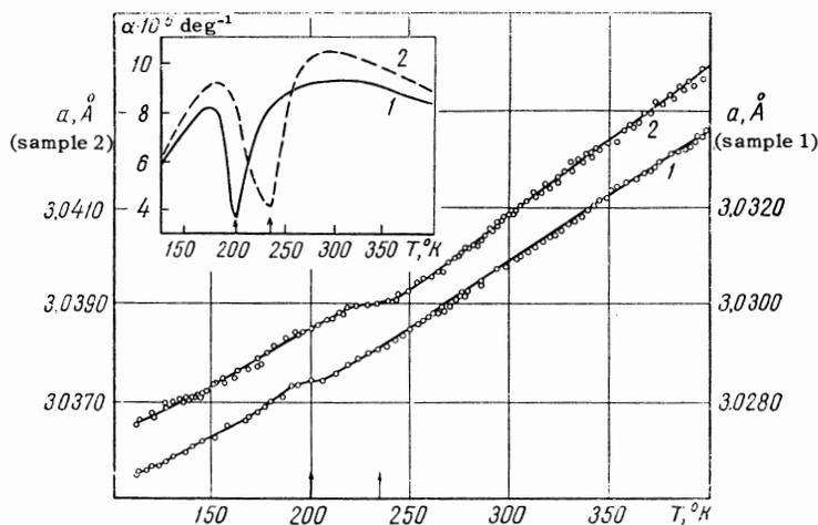
FIG. 3. Temperature dependence of the crystal lattice parameter and the linear expansion coefficient of vanadium of 99.74% purity (curves denoted by 1) and 99.20% purity (curves denoted by 2).
