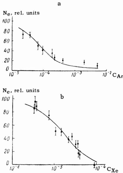
FIG. 2. Dependence of electron counting rate  $N_e$  on the concentration of atoms a - of argon, and b - of xenon, in hydrogen.
