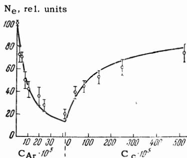
FIG. 3. Dependence of electron counting rate on the concentration of atoms of argon and, for a concentration of argon  $C_{Ar} = 4.2 \times 10^{-4}$ , on the concentration of carbon atoms.
