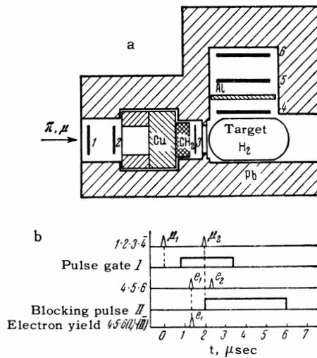
FIG. 1. Drawing of experimental apparatus (a) and time scale of the pulses (b).
