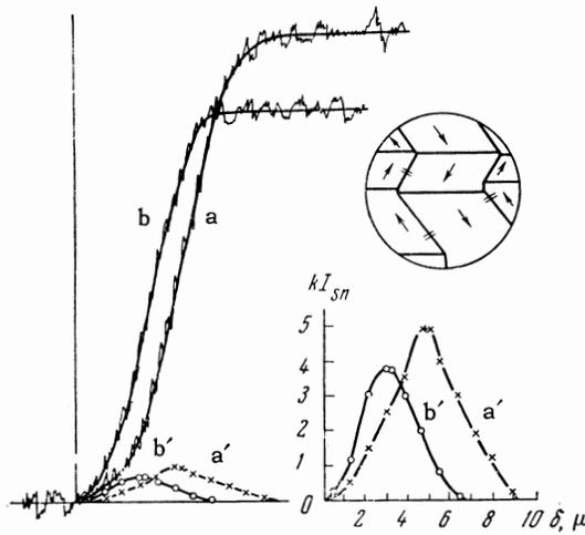
FIG. 4. Curves recorded on the recorder's chart in the investigation of the  $180^\circ$  boundaries in a (110) plane of a single crystal of the iron-nickel ferrite: a) before heat treatment; b) after heat treatment; a' and b' are the corresponding differential curves, which give the magnetization distribution in the boundaries. The schematic drawing on the right at the top of the figure shows where the boundaries were recorded.
