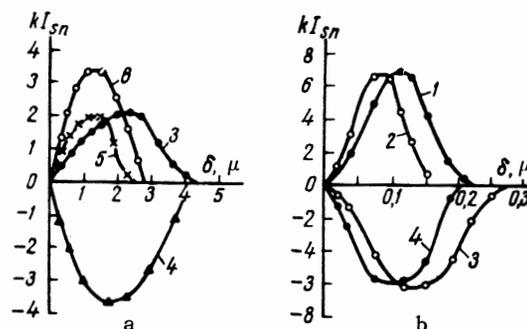
FIG. 3. Magnetization distribution in the domain boundaries of: a) iron-manganese ferrite (the numbers alongside the curves correspond to the numbers of the curves in Fig. 2); b) iron-cobalt ferrite (1 and 3 – before heat treatment, 2 and 4 – after heat treatment).
