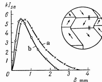
FIG. 5. Distribution of the magnetization in the  $71^\circ$  boundaries in a (110) plane of a single crystal of the iron-nickel ferrite (a—before heat treatment, b—after heat treatment). The schematic drawing on the right shows where the boundaries were recorded.
