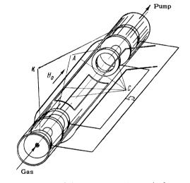
FIG. 1. Drawing of the apparatus: K = cathodes, A = anodes, C = stabilizing current conductors.
