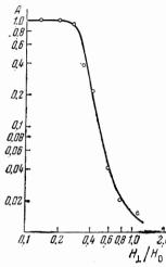
FIG. 3. Variation of the alternating component of the current to the probe with the ratio  $H \perp / H_o$ .
