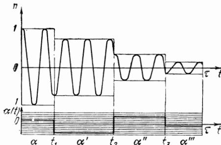
FIG. 2. Population relaxation in the interval  $(0\tau)$  for  $k = 3$ . In the lower part of the figure the shading indicates the range of possible phases; the bold line indicates its sequential changes in one realization of perturbation consistent with the indicated distribution of the times  $t_1, t_2$ , and  $t_3$ .
